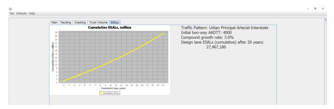
Figure 4-5 PittRigid ME screen with the results of ESALs prediction for Case 1
