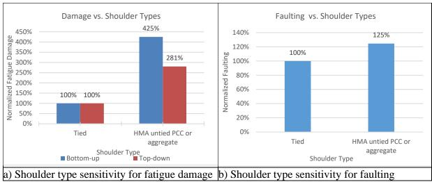
Figure A.13. Effect of should type on predicted fatigue damage and joint faulting
