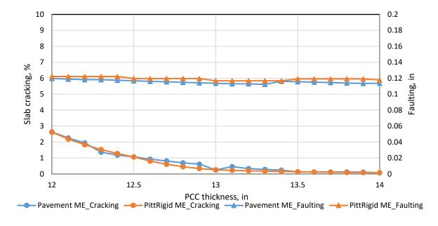
Figure 4-11. Comparing slab cracking and faulting predictions between Pavement ME and PittRigid ME at 50% reliability with respect to PCC thickness for Case 5
