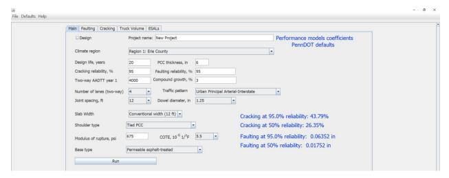
Figure 4-1. Main screen of PittRigid ME with the inputs and outputs for Case 1
