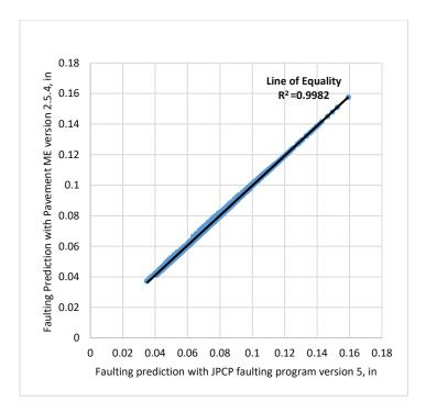
Figure 3-3. Comparisons of faulting predictions between using JPCP faulting program version 5 and Pavement ME version 2.5.4
