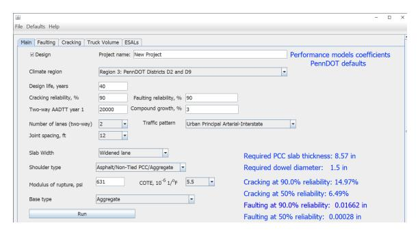
If the analysis option is not selected, only the predicted cracking at the specified reliability level, the predicted cracking at 50% reliability, the predicted mean joint faulting at the specified reliability level, and the predicted mean joint faulting at 50% reliability level are displayed.
