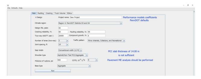
The user should either use Pavement ME software for the project or consider modification of design features, such as reduction of joint spacing, the use of a widened slab, or an increase in the modulus ruptures. For example, a decrease in joint spacing from 15 to 12 ft leads to the required PCC slab thickness of 9.82 in (see figure below). This means that this slab thickness is sufficient to meet the transverse cracking predicted performance requirement at the specified reliability level.
