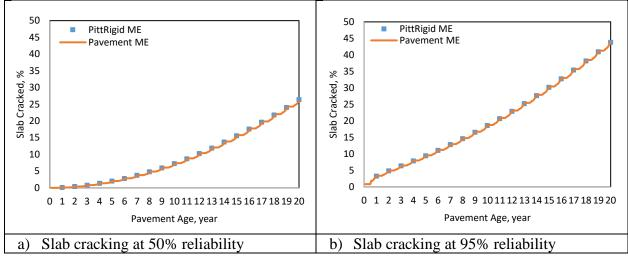
Figure 4-6. PittRigid ME and Pavement ME slab cracking prediction comparisons for Case 1
