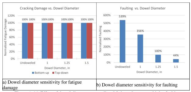
Figure A.14. Effect of dowel diameter on predicted fatigue damage and joint faulting
