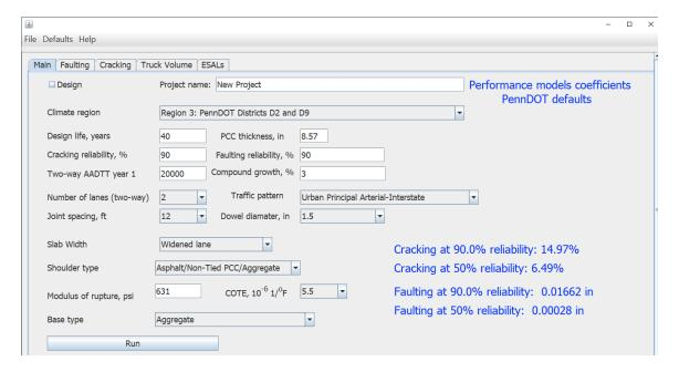
After the analysis is complete, the user can select the tabs "Faulting" or "Cracking," to view the predicted faulting and cracking, respectively.
