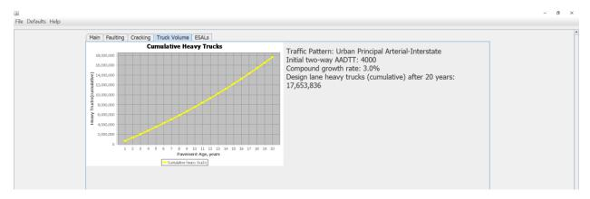
Figure 4-4. PittRigid ME screen with the results of design truck lane traffic prediction for Case 1
