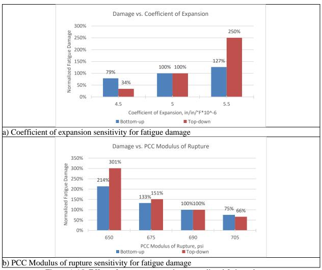
Figure A.15. Effect of concrete properties on predicted fatigue damage
