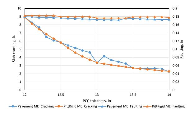
Figure 4-12. Comparing slab cracking and faulting predictions between Pavement ME and PittRigid ME at 90% reliability with respect to PCC thickness for Case 5
