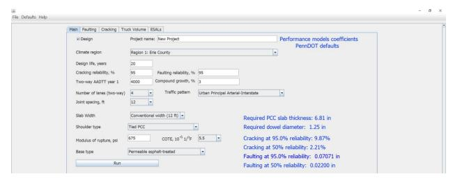
Figure 4-8. Main screen of PittRigid ME with the inputs and outputs for Case 2
