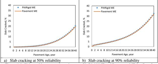
Figure 4-9. Slab cracking comparisons between PittRigid ME and Pavement ME for Case 3
