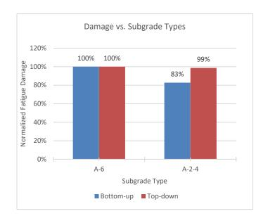
Figure A.17. Effect of subgrade type on predicted fatigue damage
