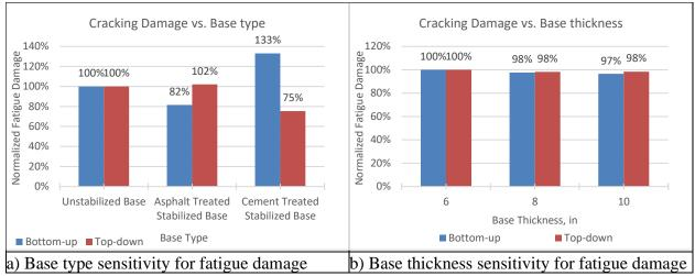
Figure A.16. Effect of base type and thickness on predicted fatigue damage
