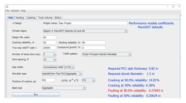
However, in this example, the predicted faulting performance does not meet the specified requirement even for the dowel diameter of 1.5 in. The use of a widened lane leads to a design solution meeting both cracking and faulting performance requirements.
