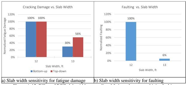
Figure A.12. Effect of PCC slab width on predicted fatigue damage and joint faulting
