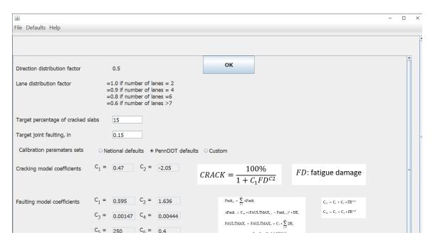
The user has an option to change the target performance criteria for slab cracking and joint faulting. By defaults, these parameters are set to 15% slabs cracks and 0.15 in mean joint faulting at the end of the design life.
